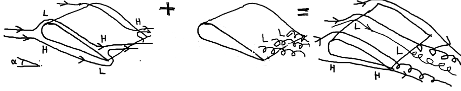
Figure 2: Stable physical 3d turbulent flow (right) with lift/drag, generated from potential flow (left) by a perturbation at separation consisting of counter-rotating tubes of streamwise vorticity (middle), which changes the pressure at the trailing edge generating downwash/lift and drag.
