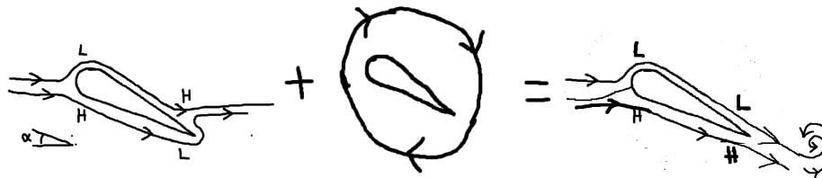
Figure 1: High (H) and low (L) pressure distributions of potential flow (left) past a wing section with zero lift/drag modified by circulation around the section (middle) to give Kutta-Zhukovsky flow (right) leaving the trailing edge smoothly with downwash/lift and a so-called starting vortex behind.
