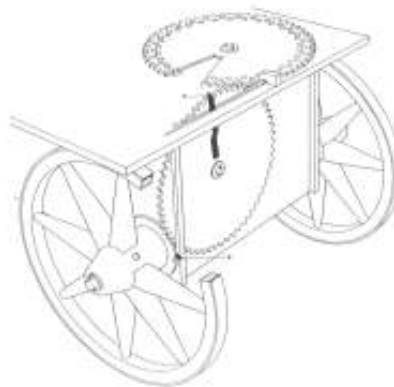
FIGURE 14.2. The hodometer was used by the Romans to measure distances, e.g. along roads. Can you figure out how it worked?.
