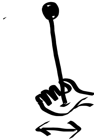
Figure 84.1: The motion of a normal pendulum is reversible, but that of a balanced inverted pendulum is not.
