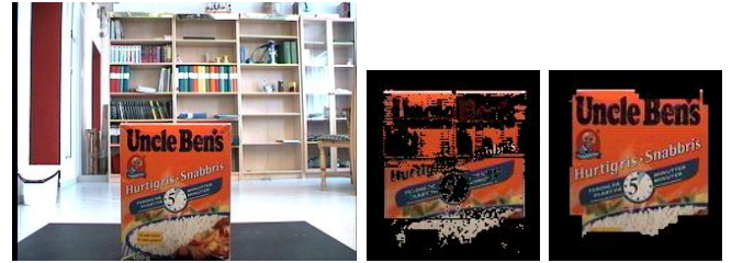
Fig. 4. Left: The original image. Center: The result after image differencing. Right: The result after morphological operations
