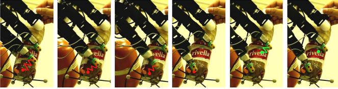
Fig. 10. The rivella bottle is grasped by the Allegro hand and a human is applying random perturbations on top of it. The red and green points are showing the new locations for fingertip  $F1$  and  $F2$  computed by Alg. 2 with virtual springs in the virtual frame.
