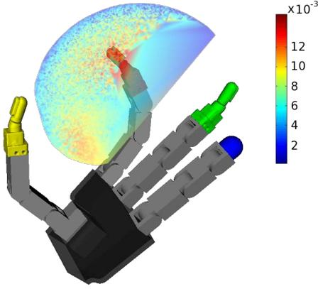
Fig. 5. Grasp Adaptability for fingertip 1. Adaptability is computed for fingertip positions sampled in joint space. The colored volume shows fingertip positions and their adaptability values.
