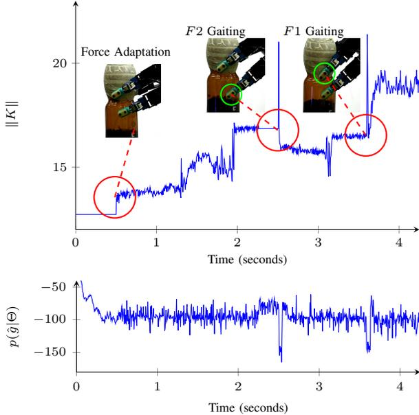
Fig. 18. A record of supported weight test of a grasp on rivella bottle. Upper: The norm of grasp stiffness and fingertip gaiting. Lower: Likelihood for grasp stability estimation defined in Eq. (18).
