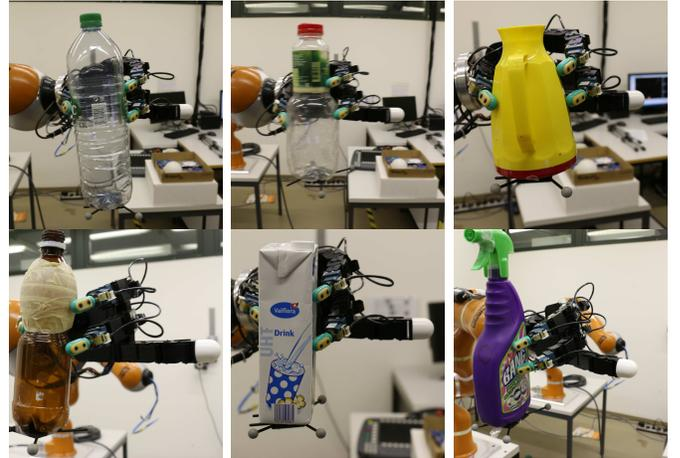
Fig. 12. Six example objects used in the evaluation: there is both variation in global geometry as well as local surface properties.
