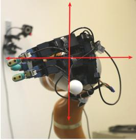
Fig. 19. The setup of grasp shaking test, in which the arm shakes each grasp in horizontal and vertical directions.  $J0$  to  $J6$  are the joint values for the initial pose of shaking test. When shaking horizontally, the shaking direction is fixed to be perpendicular to the palm.
