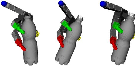
Fig. 6. Grasps with same contacts and different adaptabilities: the left grasp has the highest adaptability.
