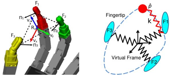
Fig. 7. Left: Virtual frame  $R_o, v_x, v_y$  and  $v_z$  defined by fingertip locations. Right: Virtual springs used by the impedance controller. A virtual spring (red) is superimposed on the impedance controller (between fingertip and the new location  $\hat{p}$ ) when a fingertip gaiting is requested.
