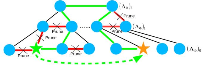
Fig. 9. Breadth-first search in *HFTS* for fingertip gaiting optimization. The green path shows how the search fringe evolves, and the red edges show the pruned path due to the 2 criteria defined in Alg. 2.
