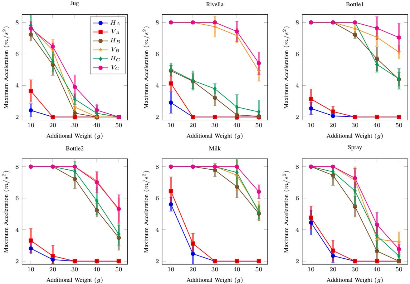
Fig. 20. Results of shaking tests on grasps shown in Fig. 12. In the legend,  $H$  and  $V$  refer to horizontal shaking test and vertical shaking test respectively.  $A$ ,  $B$  and  $C$  refer to 3 grasp strategies: grasp without adaptation, grasp adaptation in [9] and the grasp adaptation proposed in this paper.
