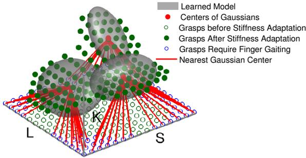
Fig. 8. GMM model  $\Theta$  for grasp stability estimation and decision making for grasp adaptation. The gray ellipsoids depict the Gaussian components of  $\Theta$ , dots and circles show grasps, represented by  $K, L, S$  in different stages, and the red lines illustrate how grasps are switched between different stages by grasp stiffness adaptation and fingertip gaiting.
