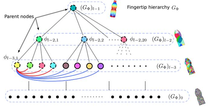
Fig. 4. Surrogate models represented as a graph. Fingertip unit partitions are represented as nodes in different levels of the hierarchy and the connectivities in this graph are represented by edges. Extra connectivities defined by Eq. (3) are exemplified in level  $l-3$  for  $\phi_{l-3,1}$ , with red edges for 2 hops and blue edges for 4 hops.
