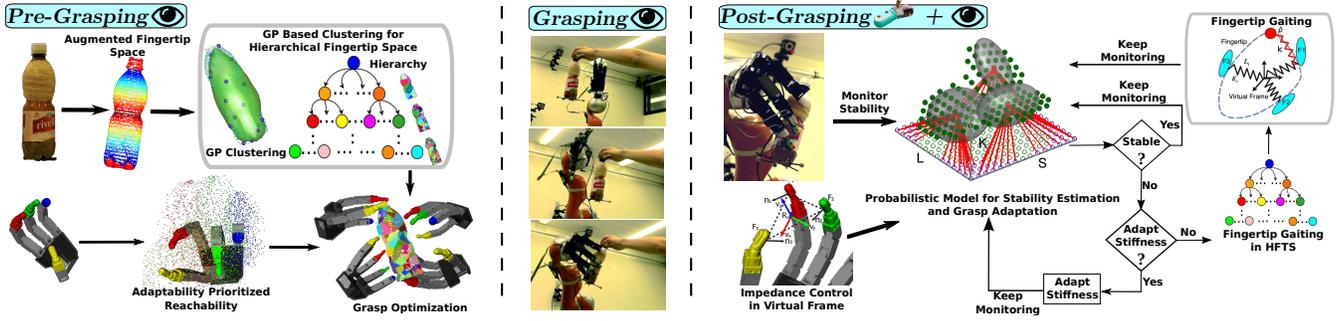
Fig. 2. Schematic overview of the system: *Pre-grasping*: After the Hierarchical Fingertip Space is generated, grasps are synthesized by a multi-level refinement strategy. *Grasping*: The synthesized hand configuration is used to execute the grasp. *Post-grasping*: Once tactile feedback is available, grasp stability is monitored by a learned probabilistic model. If a grasp is estimated as unstable, the stability is maintained through force adaptation or finger gaiting.
