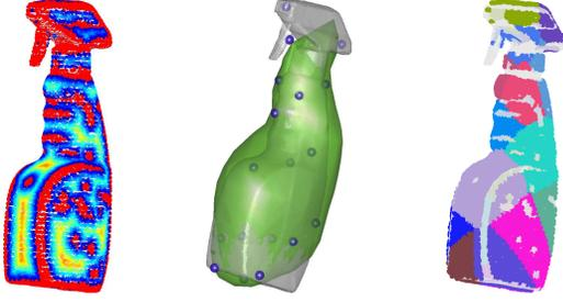
Fig. 3. Left: Fingertip Space with attached penalties rendered by jet colormap, in red are points that have been filtered out by Eq. (1), note that there are perception noise in planar areas. Middle: GP for the spray model represented by 20 cluster centers. Right: partitions of fingertip units rendered with different colors.
