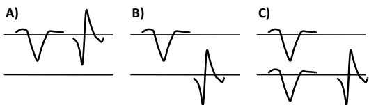
Fig. 2. Effect of spike waveform on the quality measure. A Both waveforms have their energy on the same channel yielding a low quality. B The energy of the two waveforms is unequally distributed among the channels which is rewarded by Q^{stereo} . C This combination has the highest quality, since the increase in SNR exceeds the loss in stereo effect.
