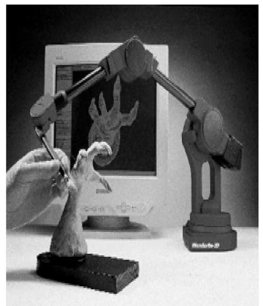
Fig. 5. We have used a MicroScribe 3D device to track position and orientation in real time.
