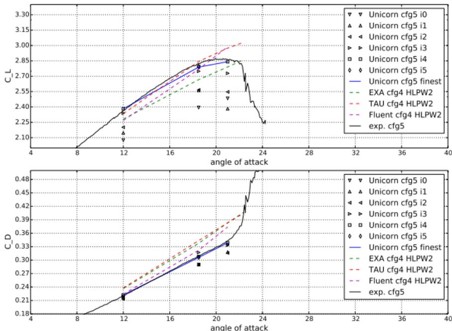
DFS/Unicorn/FEniCS consistently  $\sim 2\%$  error and reliable prediction of separation. For new config. we expect low predictive capability of Exa/RANS,  $\sim 10\%$  error and no separation prediction.
