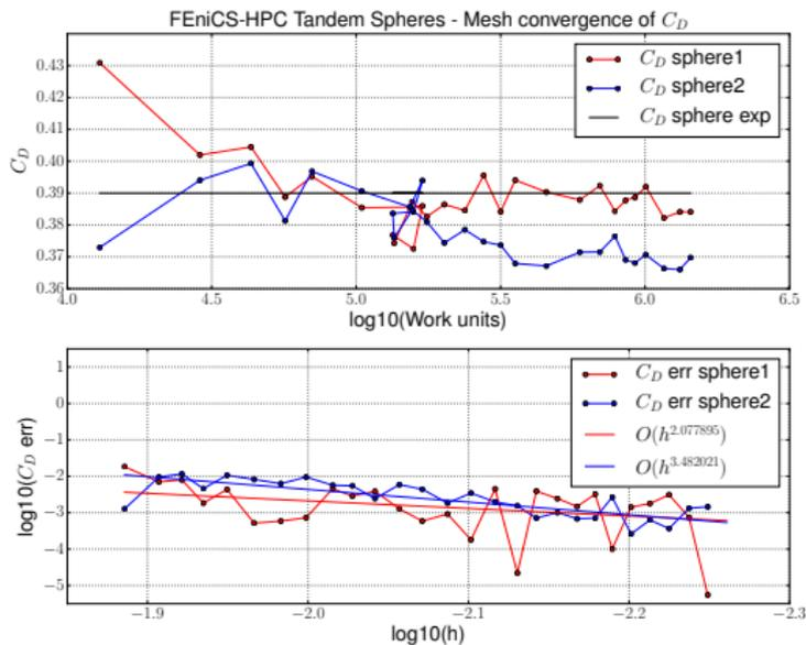
Mesh convergence of the drag coefficients of the two spheres.
