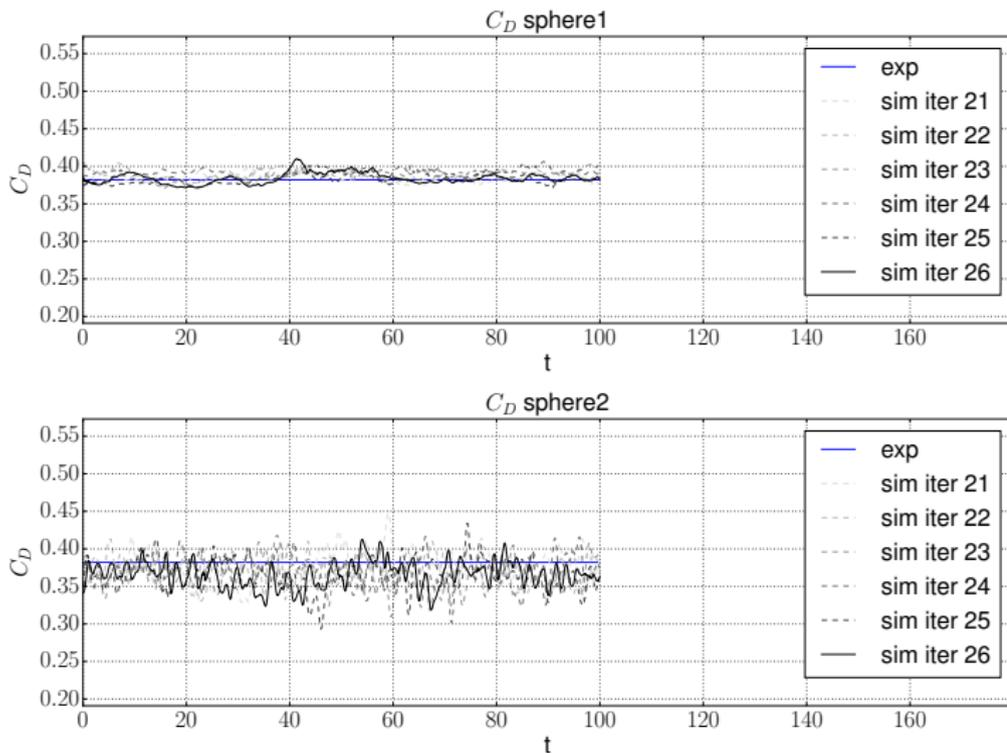
Time evolution of the drag coefficient for various iterations of our adaptive procedure.
