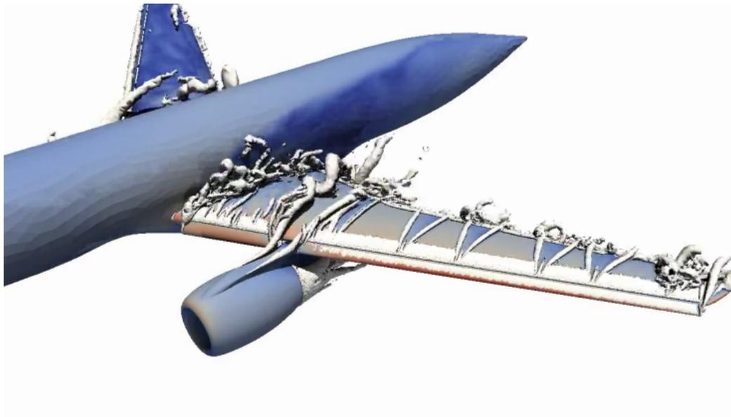
Direct automated/parameter-free prediction of new configuration - best possible simulation at given cost
