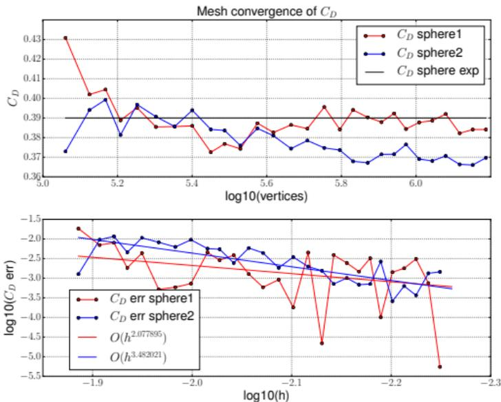
Mesh convergence of the drag coefficients of the two spheres. Effective order of convergence  $> 3$ . However, not interesting with asymptotic behavior. Allowing coarsening could give different behavior, (Couchman/Galbraith).
