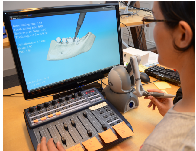
Figure 1. Designer using a PHANTOM Omni device and MIDI controller interface to sketch the material properties of a dental anatomy exploration application
