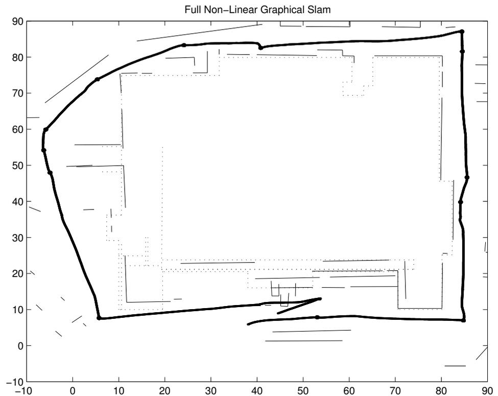
Figure 6.4: Here is a map made using the exact nonlinear energy for the system. The robot slid sideways at one point which caused the error in closing the loop. We see that the data association problems are now not present.
