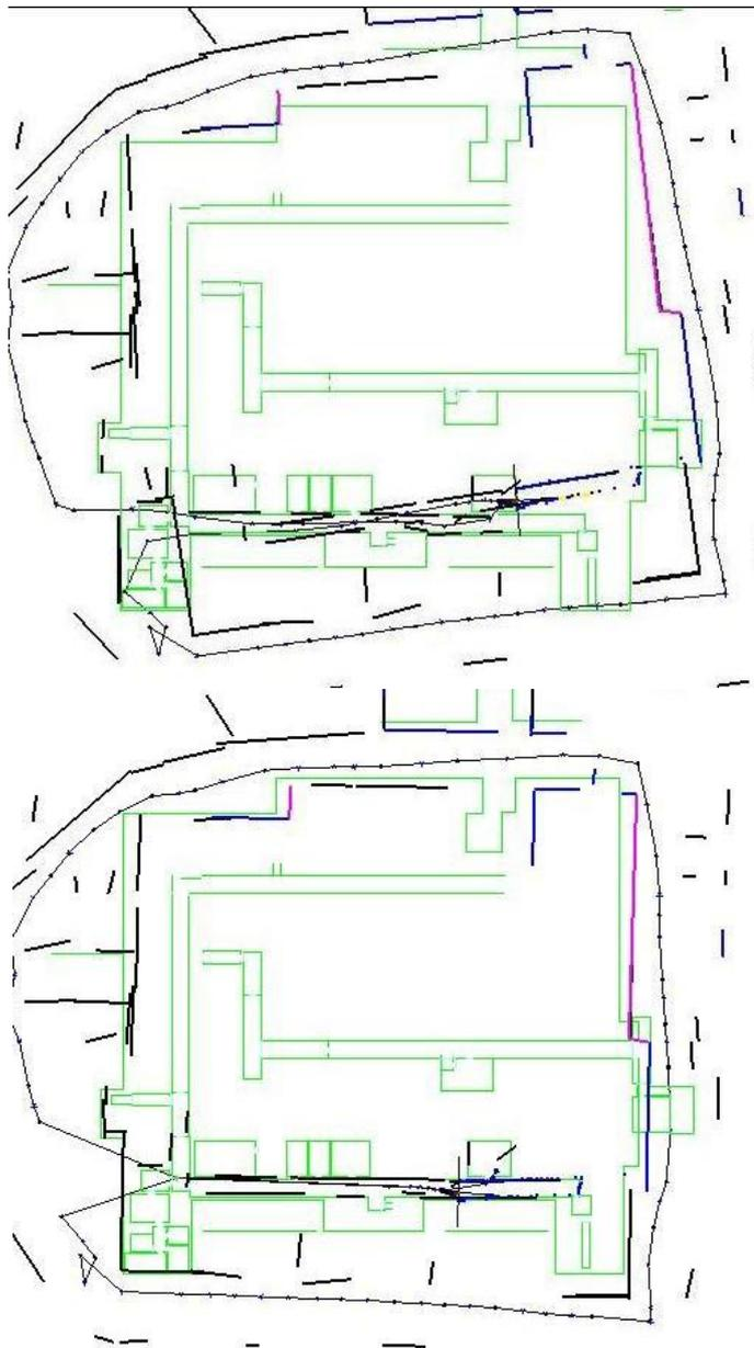
Figure 6.15: The 1<sup>st</sup> loop closing, just prior, top and after, bottom. The loop closing is done on a section of the graph with enough mature features to make multiple matches possible. The match is made between features near the bottom left corner both indoor and outdoor walls.
