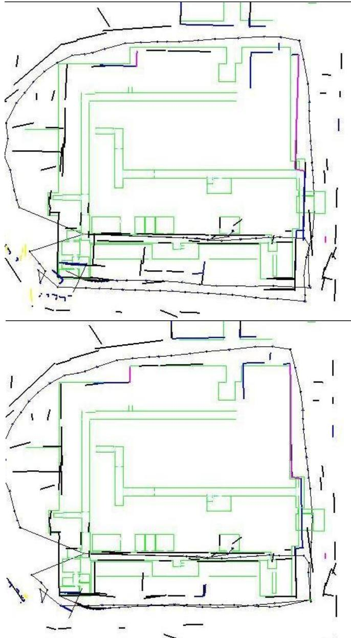
Figure 6.16: The 2<sup>nd</sup> loop closing, just prior, top and after, bottom. the outdoor section in the bottom right corner of the building is used to set the constraint.
