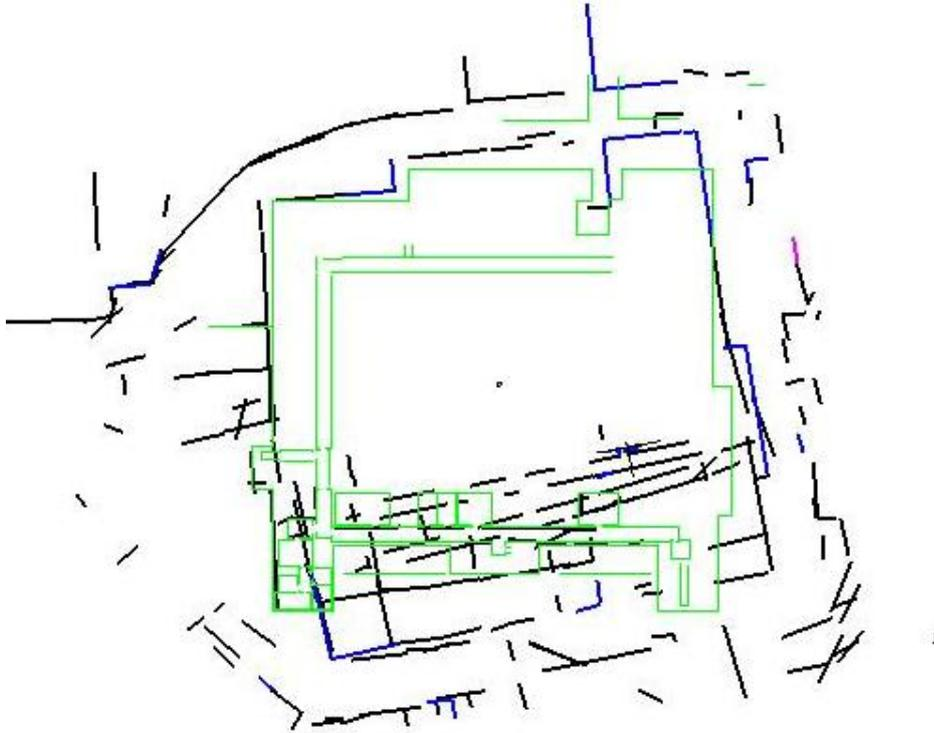
Figure 5.11: Here we show the EKF solution to a data set with 3 closed loops. The algorithm again has no way to deal with the large errors that have accumulated around the loops. The size of this area is about 100 x 100 m.
