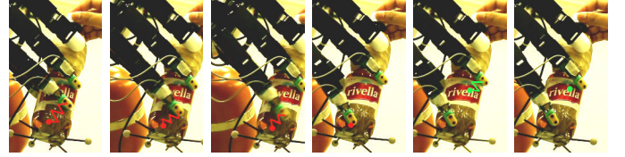
Fig. 10. The rivella bottle is grasped by the Allegro hand and a human is applying random perturbations on top of it. The red and green points are showing the new locations for fingertip F1 and F2 computed by Alg. 2 with virtual springs in the virtual frame.
