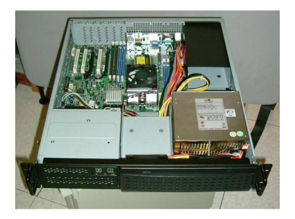
AMD Opteron 2356 with one quad core 2.3GHz Barcelona CPUs on a TYAN 2927 Motherboard (2U)
