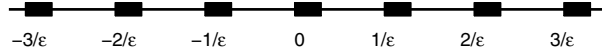
FIG. 2. The R_b^\epsilon projection. Solid rectangles have width 2b and correspond to the pass region in frequency space.
