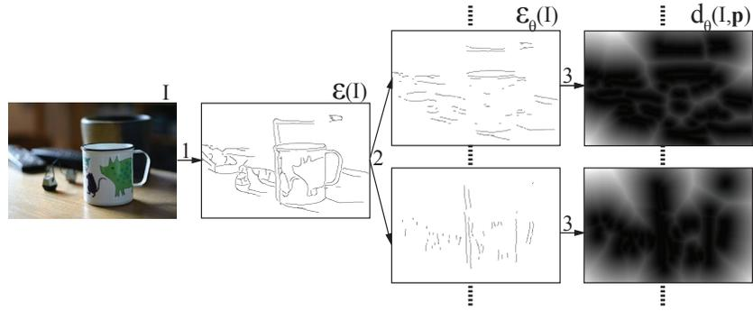
**Fig. 4.** Images are preprocessed as follows: (1) extract a set of oriented edges  $\mathcal{E}(I)$ , (2) split  $\mathcal{E}(I)$  into (overlapping) subsets  $\mathcal{E}_\theta(I)$  and (3) compute the distance transforms  $d_\theta(I, \mathbf{p})$ .
