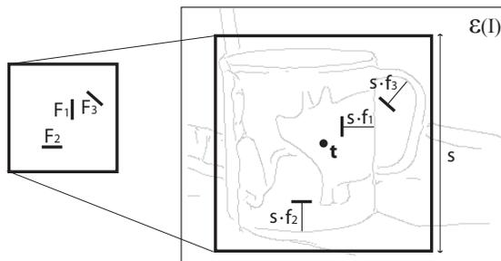
**Fig. 3.** Feature values  $f_k(I, \mathbf{t}, s)$  are computed by translating ( $\mathbf{t}$ ) and scaling ( $s$ ) features  $F_k = (\mathbf{x}_k, \theta_k)$  and taking the (normalized) distances to the closest edges with similar orientations in the image.
