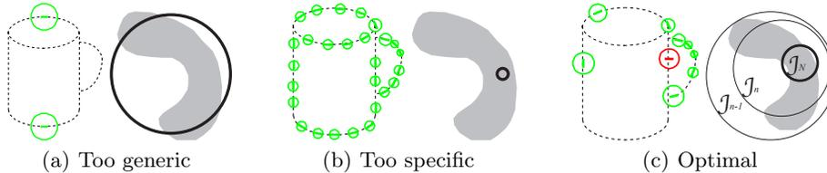
**Fig. 5.** The number of single feature classifiers controls the specificity of a weak classifier. a) Using too few yields weak classifiers that are too generic to delineate the class manifold (gray). b) Using too many yields weak classifiers that are prone to overfitting and that are inefficient at representing the class. c) We learn the optimal number of single feature classifiers for each weak classifier (the notation is defined in the text).
