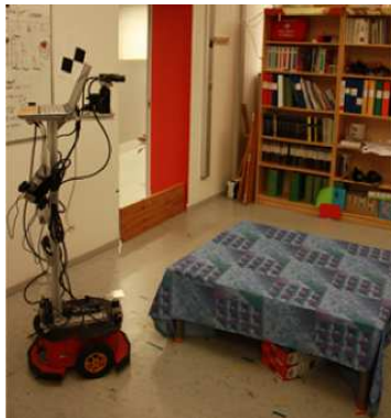
Figure 5. Chained inference, direct search: While searching for the rice carton, the robot looks towards the height of the target object had it been on top of the large box object.
