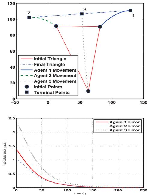
Fig. 5. The motion of a triangular formation consisting of three mobile agents starting in a random triangle and given a desired collinearity condition.
