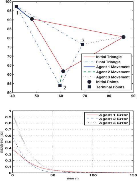
Fig. 3. The motion of the formation with a desired terminal constraint of  $\alpha_1^* = \pi/6$ ,  $\alpha_2^* = \pi/4$  and  $\alpha_3^* = 7\pi/12$ .
