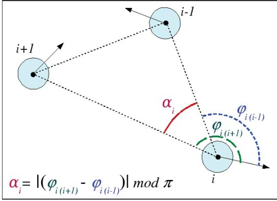
Fig. 1. Agent  $i$  computes  $\alpha_i$  from the bearing measurements taken in a local coordinate system.
