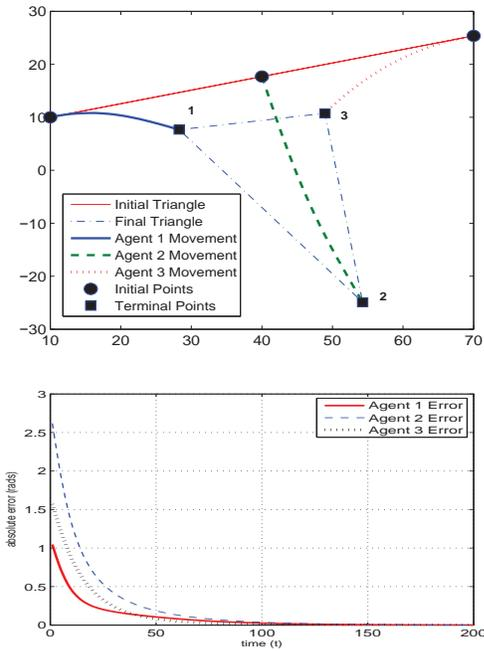
Fig. 4. The motion of a triangular formation consisting of three mobile agents initially in a collinear position with desired terminal constraints  $\alpha_1^* = \pi/3$ ,  $\alpha_2^* = \pi/6$  and  $\alpha_3^* = \pi/2$ .
