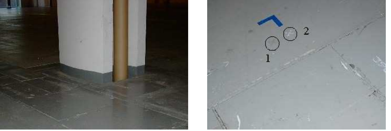
Figure 15: An example of how a foreign obstacle can cause marking errors. Left: images shows how a paper tube has been leaned against a pillar. Right: The resulting marks with and without the tube present are circled and denoted 1 and 2 respectively. Mark 2 is very close to correct and the error for 1 corresponds to the size of the tube. The manual mark is also shown next to the two circles. This mark is more incorrect in absolute sensor then both of the automatic marks.
