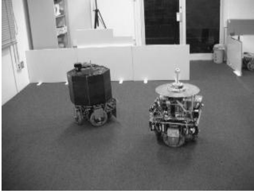
Figure 4.9. The black robot has allocated the paths' intersection and the white one has to wait.
