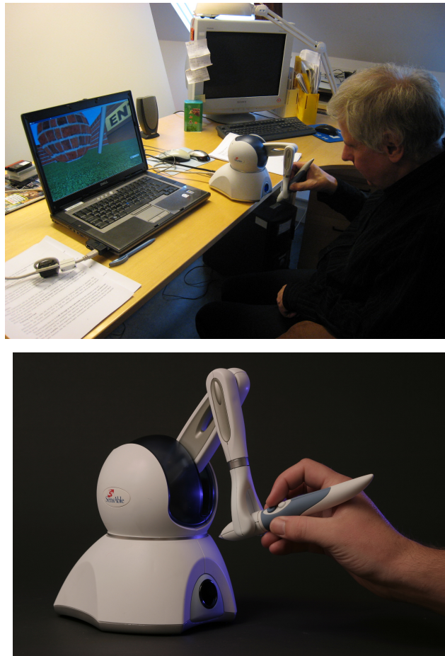
Fig. 21. Experiment setting on the left and one Phantom Omni force feedback device on the right (source: SensAble Technologies Inc).
