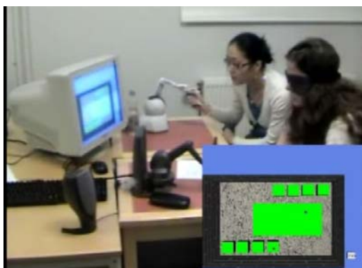
Fig. 1. Experimental setup. The two participants (the one closest to the camera is blindfolded) are seen holding one PHANTOM device each.
